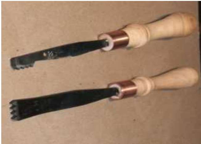
Figure 1. A pair of hand chasers (top) inside chaser and (bottom) outside chaser. These chasers are for 4.5 tpi threads.
